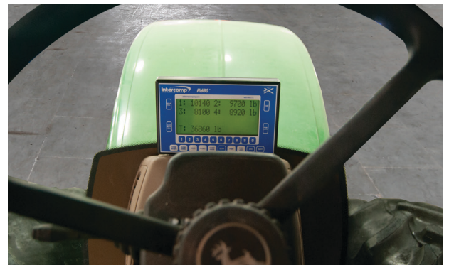
Built-in RFX™ Wireless Weighing capability allows up to six scale pads to communicate with a wireless handheld indicator.
